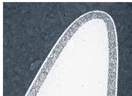
Cross section of the wire tooth with 3M™ Wear Protection Coating
