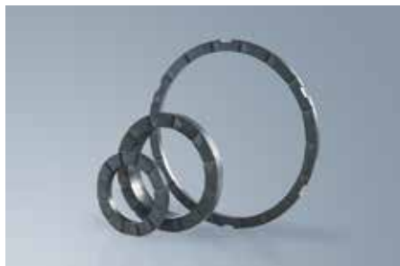
3M™ Silicon Carbide laserstructured Sliding Bearings (left: radial bearing, right: thrust bearings) used e.g. in highly-loaded chemical pumps, in magnetic couplings for hermetically sealed pumps and in stirrers for chemical and pharmaceutical processes.
