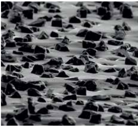
Structure of 3M™ Friction Shim
